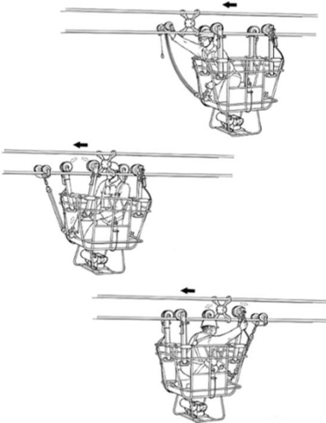
*Figure 4: Spacer trolley*
