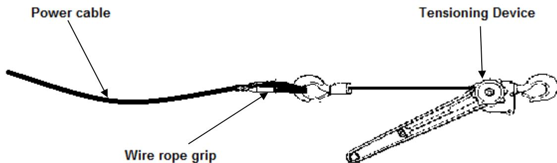
**Figure 1: Tensioning assembly**
